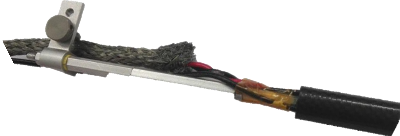
Figure 1: Custom made 11mm rodent sTMS coil
